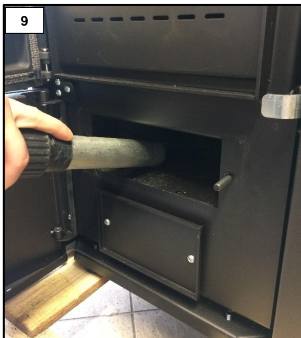
Vacuum any residues inside the ash box compartment (Figure 9).
