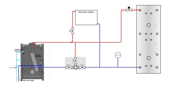
Below is a typical schematic showing connection to an open vented system with a thermal store. Again care and attention should be paid to how, and where, the heat leak radiator, and fill and expansion tank are connected.
